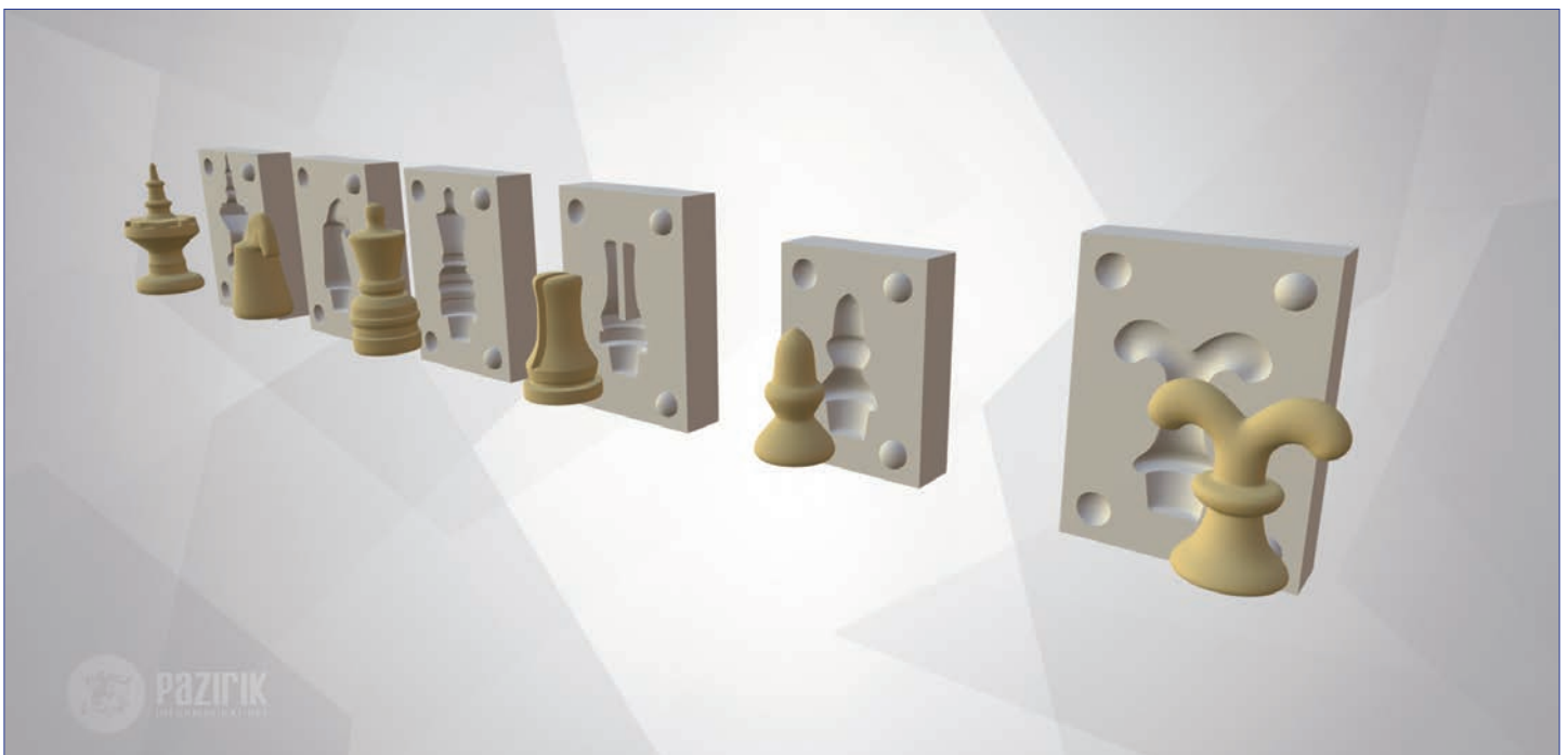
Fig. 4 — The virtual 3D-modeling of the press-moulds.
